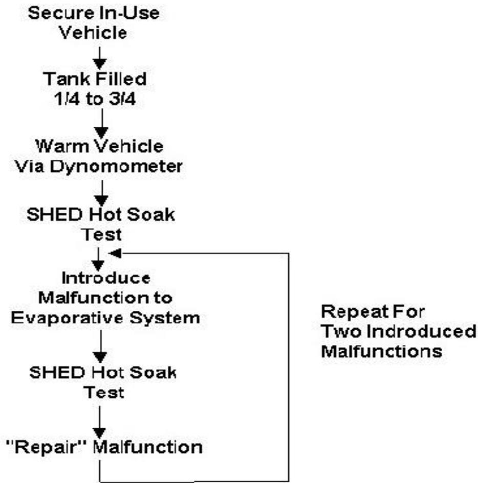
Figure 1. Methodology of emissions evaporation measurement testing.
