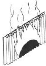
Figure 3. Vertical Flame Spread Helped by Convection
